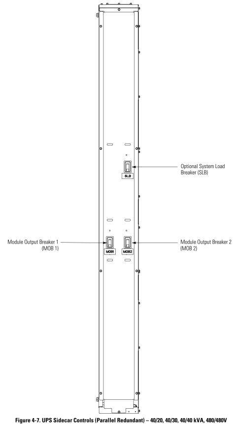
jure 4-7. UPS Sidecar Controls (Parallel Redundant) – 40/20, 40/30, 40/40 kVA, 480/48 with MOBs and Optional SLB
